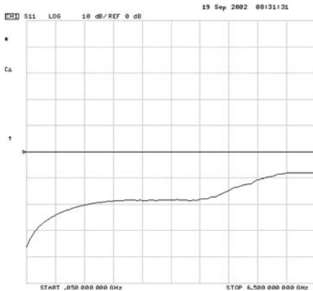
Return loss tested to 6.5 GHz for the CRF Reed Relay. Horizontal full scale: 6.5 GHz. Vertical scale: 10 dB/div referenced from the 0 mark.
