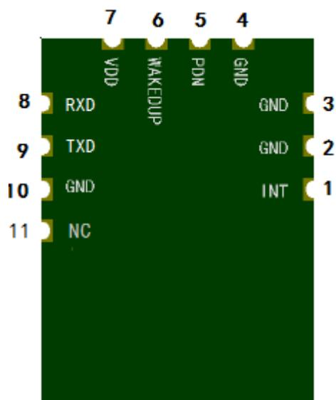
Fig. 3. Module Pins Distribution Diagram (Bottom View)
