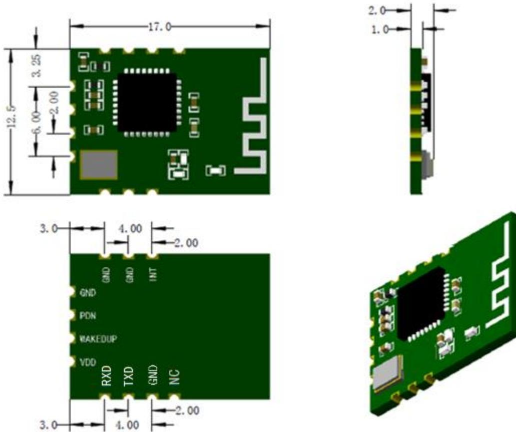
Fig4. Module Size Diagram
