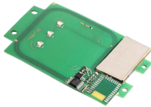
TWN4 MultiTech 2 HF PCB top view
