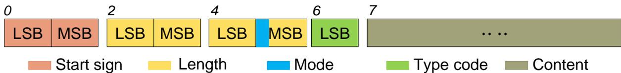
FIG 3 YDLIDAR G4 SYSTEM MESSAGE DATA PROTOCOL
