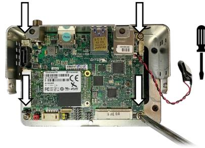
**Step 9:** Thread the power button cable through the hole for the power button. Plug the cable into the front panel connector (CN3 in user manual). NOTE: The white dot indicates PIN 1 connector, make sure the connector is properly aligned. Next, gently push the power button in until it is secure (you will hear a 'snap'). Be careful not to tangle the power button cable with the CMOS battery cable.
