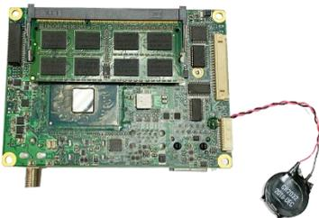
**Step 5:** To install m.2 storage module, remove the securing screw.
