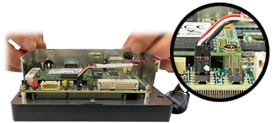
**Step 10:** Peel the backing off of the tape on the CMOS battery. Gently press the battery onto the PICO-APL1 board to secure it.
