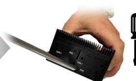
**Step 13:** Replace the washer and nut for the power input port.
