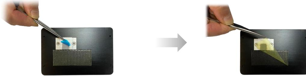
**Step 2:** Place the top chassis onto the heatsink. Note the orientation of the chassis with the heatsink. Secure with four black screws.
