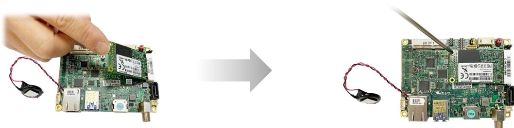
**Step 7:** Insert the PICO-APL1 board into the chassis assembly with the processor side toward the heatsink. DO NOT place the CMOS battery between the board and heatsink.
