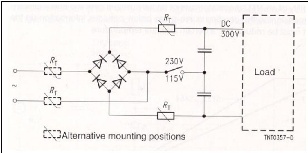
**Fig.2 Possible locations of NTC for inrush current limiting**
