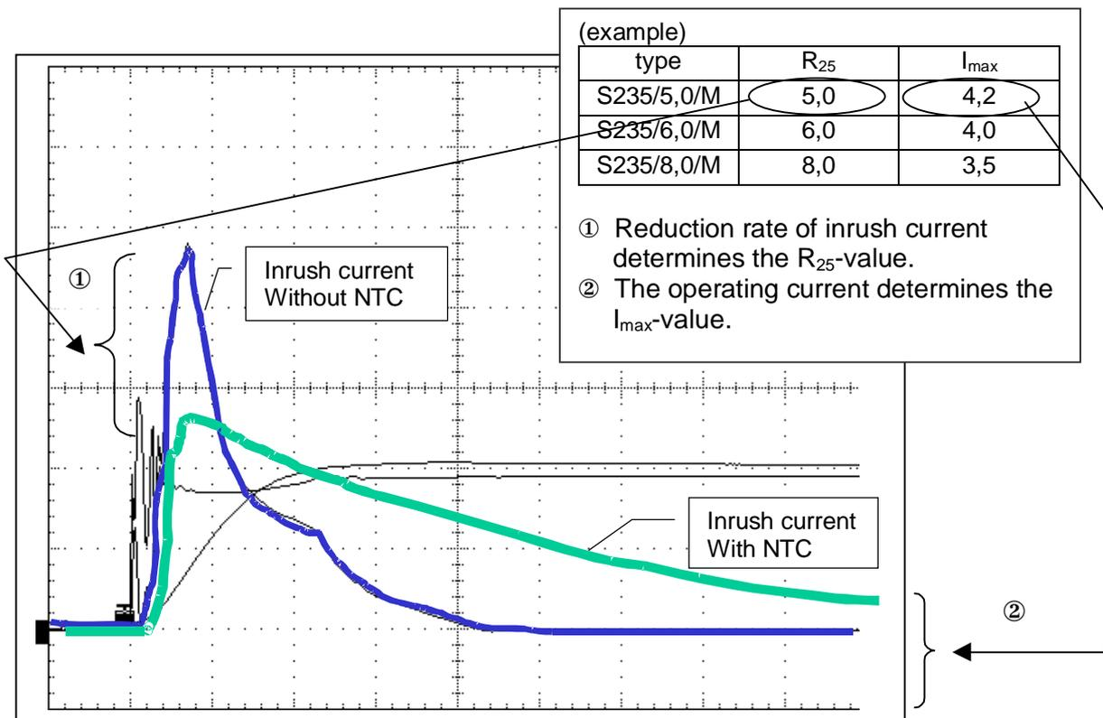
**Fig.3 Typical current characteristic in load after turning on**
