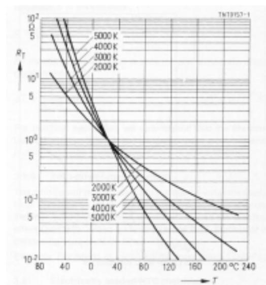
**Fig.1 R/T characteristics (parameter :B value)**
