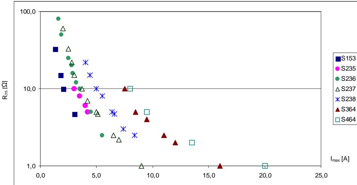
**Diagram 1: Selection criteria for the inrush current limiter : resistance at 25°C and rated current**
