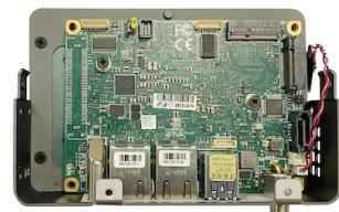
**Step 6:** Check that the I/O ports are properly aligned. Secure board with four nickel screws.
