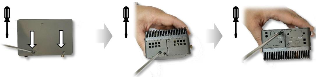
**Step 11:** Replace the washer and nut for the power input port.
