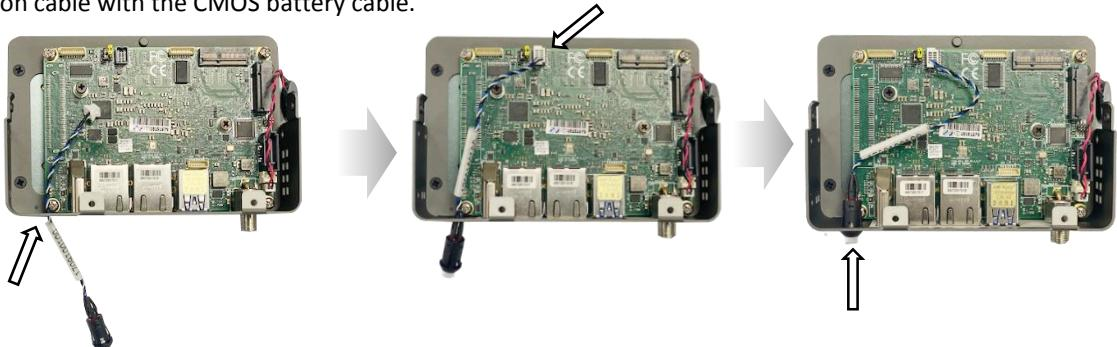
**Step 8:** Peel the backing off of the tape on the CMOS battery. Gently press the battery onto the PICO-KBU4 board to secure it.
