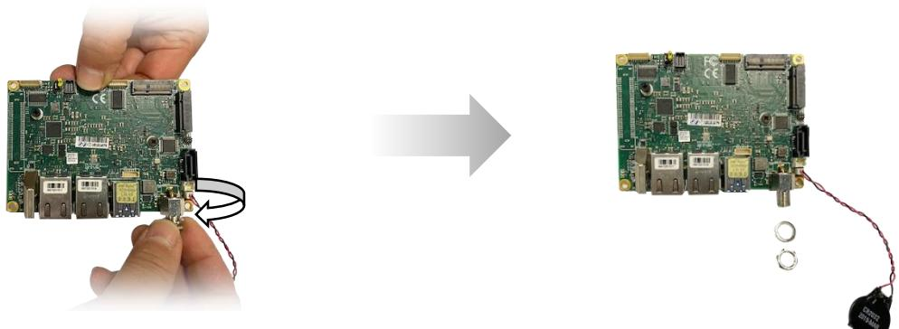
**Step 4:** Connect the thermal fan cable to the PICO-APL4 board as shown.
