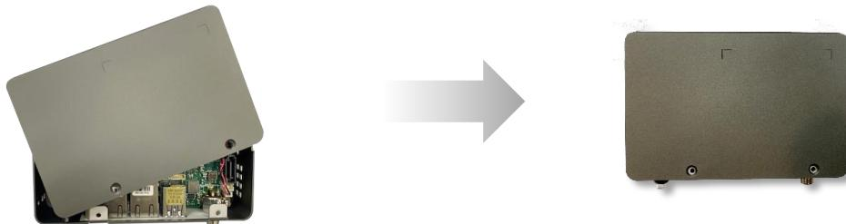
**Step 10:** Ensure the bottom chassis is properly lined up and attached. Use black screws to secure, two screws on the bottom and one screw on the left and right sides of the chassis.
