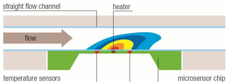
Due to the small size of the sensor chip and the very thin flow channel wall ( $\leq 100 \mu\text{m}$ ), even the slightest deposition can cause measurement deviations. Depending on the kind of deposits, a few micrometers might be sufficient to cause considerable measurement deviations. These deposits may be permanent (i.e. mineral or salt deposits) or transient (layer of previous liquid among alternating media types).
