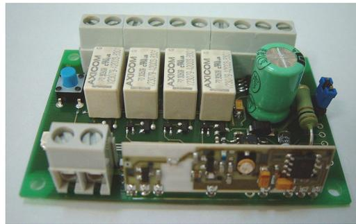
The decoder board HCS-DEC-4 is a 4 channels central unit which can be matched with any HCS Keeloq encoded keyfob programmed with Aurel manufacturer code.
