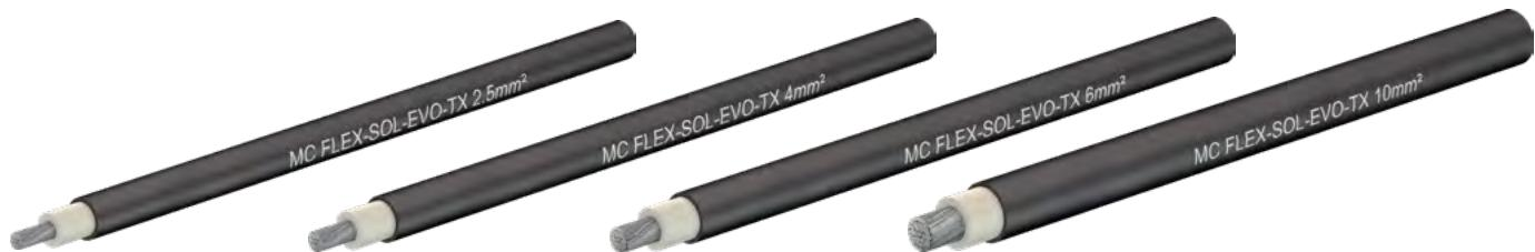
Halogen free, low smoke, flexible, single-core, cross-linked double layers photovoltaic cables, in particular for use at direct current (DC) side of photovoltaic systems. These cables are designed to match with most PV components according to class II with a nominal DC voltage of 1.5 kV (IEC) between conductors and between conductor and earth. The maximum permitted operating DC voltage is 1.8 kV.
