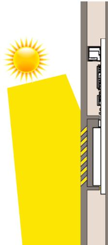
**Figure 8:** Cross-sectional view: sun protection through an angled aperture design.
