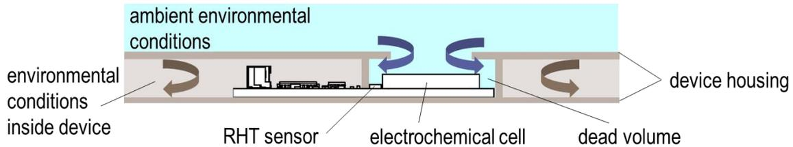
**b) Decoupling from external heat sources**
