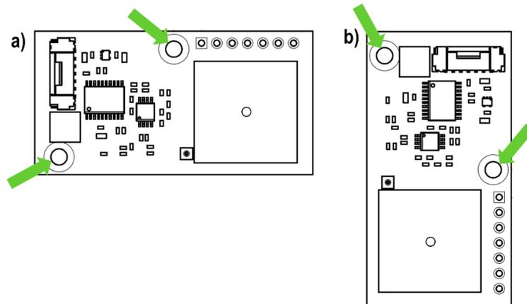
**Figure 5:** Mechanical mounting (two mounting holes indicated by green arrows) and recommended orientation of SFA30 sensor module with the Molex connector facing (a) sideways and (b) upwards.
