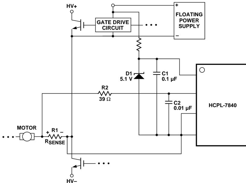
Figure 17. Recommended Supply and Sense Resistor Connections.
