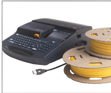
ProMark MK9-USB Bench top machine for on site marking with Partex ProMark system. For further information see separate product information.
