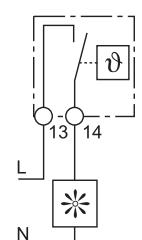
**Heating control** - Should the panel temperature fall below the (minimum) set temperature the contact will close to call for heat. The contact will open when this set temperature is exceeded.
