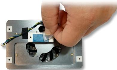
**Step 2:** Place the top chassis onto the thermal assembly. Note the orientation of the chassis with the thermal assembly. Secure with four black screws.
