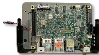
**Step 7:** Check that the I/O ports are properly aligned. Secure board with four nickel screws.
