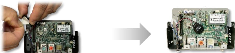
**Step 11:** Attach the bottom chassis by first lining up the right side, then swivel the chassis into place. NOTE: the bottom chassis does not slide directly on, it must swivel into place as shown in the figure.
