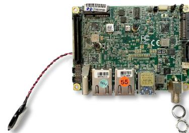
**Step 4:** On the processor side of the PICO-KBU4 board, install the memory RAM module. Insert at an angle (~30°) and then gently press down until it is secured in place.
