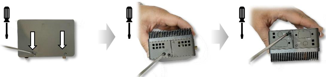
**Step 13:** Replace the washer and nut for the power input port.
