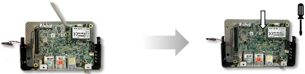
**Step 9:** Thread the power button cable through the hole for the power button. Plug the cable into the front panel connector (the 2nd connector from the front, CN15 in user manual), then gently push the power button in until it is secure (you will hear a 'snap'). NOTE: Be careful not to tangle the power button cable with the CMOS battery cable.
