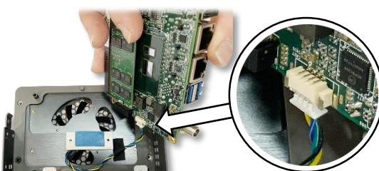
**Step 6:** Insert the PICO-KBU4 board into the chassis assembly with the processor side toward the thermal assembly. DO NOT place the CMOS battery between the board and thermal assembly.
