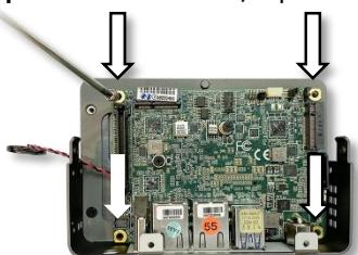
**Step 8:** To install m.2 storage module, first remove the securing screw. Insert the m.2 module at an angle (~30°). Press down gently and secure with screw.
