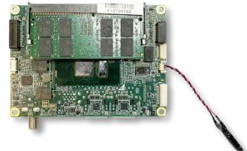
**Step 5:** Connect the thermal fan cable to the PICO-KBU4 board as shown.
