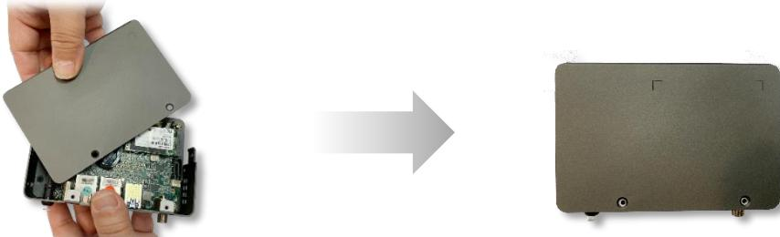
**Step 12:** Ensure the bottom chassis is properly lined up and attached. Use black screws to secure, two screws on the bottom and one screw on the left and right sides of the chassis.
