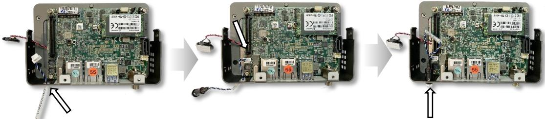
**Step 10:** Peel the backing off of the tape on the CMOS battery. Gently press the battery onto the PICO-KBU4 board to secure it.
