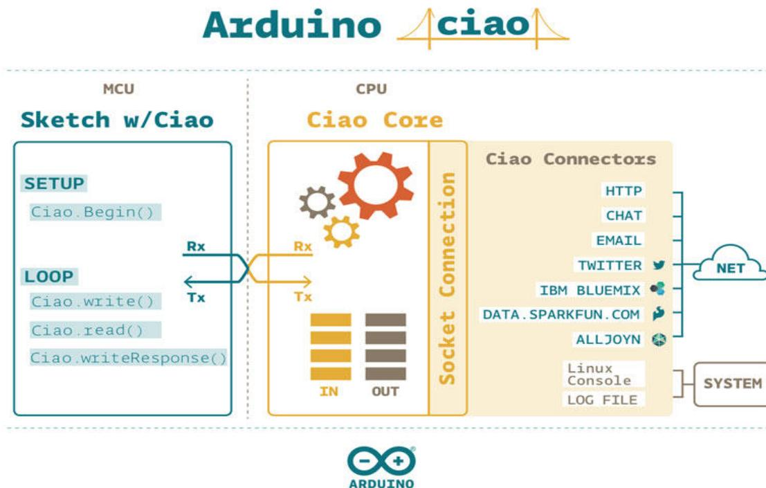
Arduino Ciao is an easy-to-use and powerful technology that enables Arduino sketches to communicate intuitively with the "outside World". It aims to simplify interaction between microcontroller and Linino OS, allowing a variety of connections with most common protocols, third-party services and social networks.
