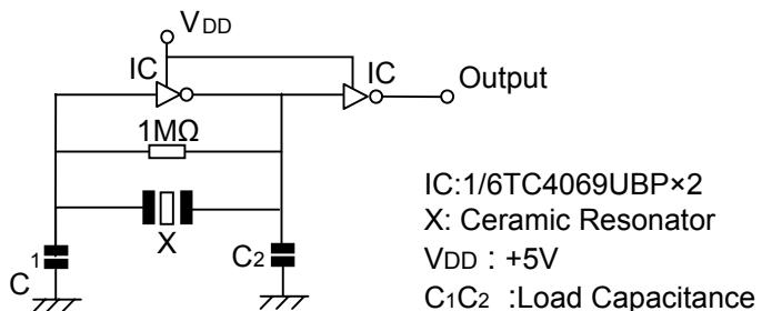
**Feedback Resistor (R = 1MΩ):**
