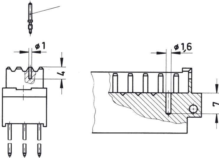
To avoid cross-plugging of adjacent connectors a coding system is required. With the aid of the marked indents between the contact rows of the male connector a hole has to be drilled at the desired position (also see drawing). The code pin can then be inserted into the corresponding cavity of the female connector by the means of the insertion tool.
